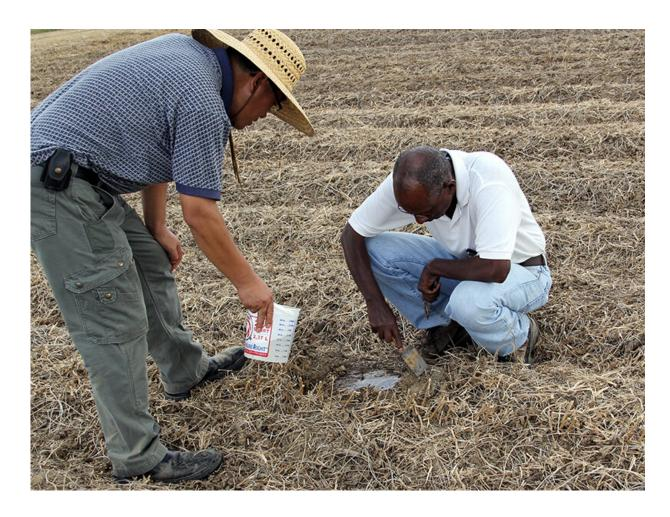
Scientists Gary Feng and Haile Tewolde test how fast water can infiltrate into soils that were fertilized by commercial inorganic fertilizer and manured by poultry litter. Credit: Gary Feng
