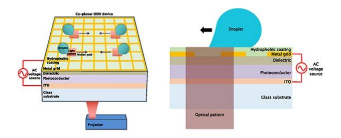
Light is selectively illuminated on the photoconductor layer under part of a droplet's contact line to achieve an electromechanical force imbalance within the droplet. This causes the droplet to move toward the light pattern. Credit: Jodi Loo et al. doi: 10.1117/1.JOM.1.3.034001.
