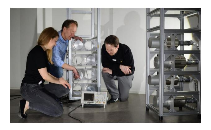
Researchers, from left, Jana Petrovic, Bo Cederwall and Alf Göök test the new imaging technology on a mock-up of radioactive waste drum scanner. Credit: Biswarup Das
