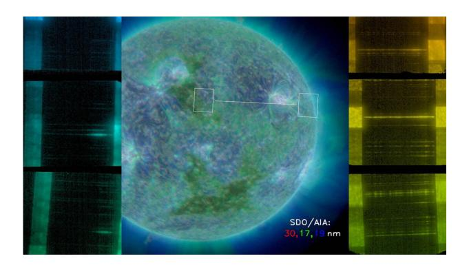
During its 2013 flight, NASA's EUNIS sounding rocket examined light from the Sun in the area shown by the white line (imposed over an image of the sun from NASA's Solar Dynamics Observatory) then separated the light into various wavelengths (as shown in the lined images—spectra—on the right and left) to identify the temperature of material observed on the Sun. The spectra provided evidence to explain why the sun's atmosphere is so much hotter than its surface. Credit: NASA/EUNIS/SDO
