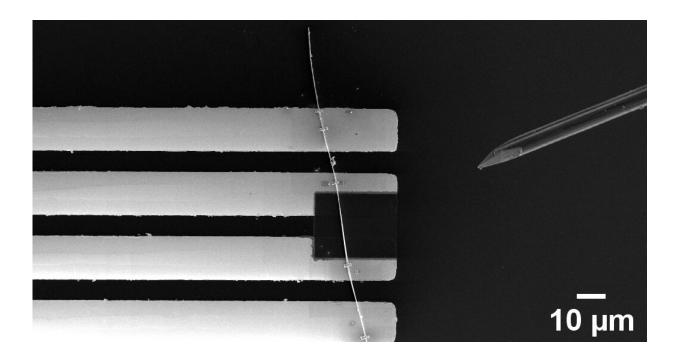
Scanning electron microscopy (SEM) image showing an example of a nanofabricated single-element device used for the gas sensing measurements. The nanostructure was nano-manipulated onto gold electrodes inside a Dual-Beam (Scanning electron microscope/Focused Ion Beam) microscope. Small platinum pads were done via electron beam induced deposition (Pt-EBID), and ensured an electrical contact between the gold electrodes and the nanobelts. Credit: University of Surrey
