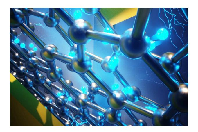
Artistic representation of the nanoscopic structure of one of the new MIT nanodevices. Two twisted sheets of graphene are represented by the metallicblue carbon atoms in a honeycomb lattice. Electrodes (gates) above and below the graphene are represented in gold. Electrons are represented by the smaller light-blue circles. Credit: Ella Maru Studio
