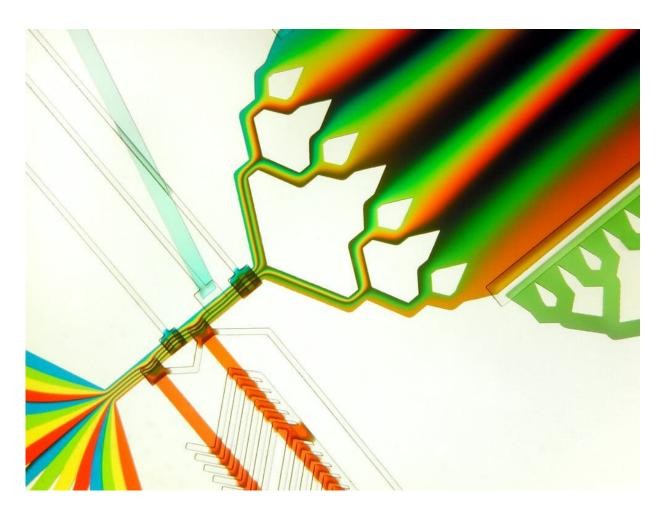
The colored liquids enter from the bottom left, but due to laminar flow, remain relatively unmixed even though they pass through one single channel and exit on the top right. Credit: Greg Cooksey and Albert Folch
