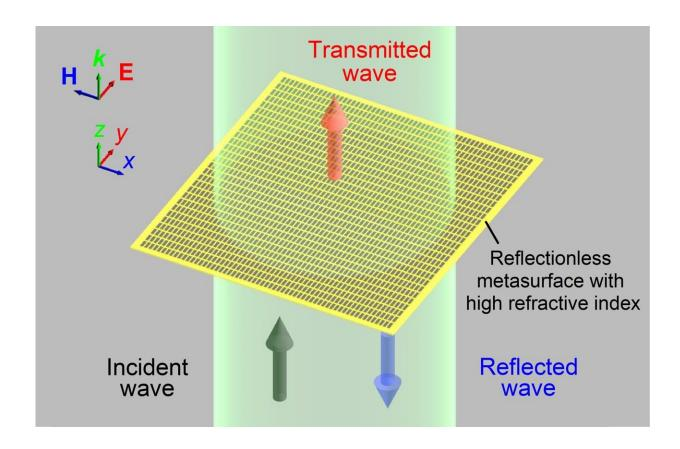
Researchers from Tokyo University of Agriculture and Technology successfully tested reflectionless, highly refractive index metasurfaces that may eventually be used in practical applications to send, receive, and manipulate light and radio waves in the terahertz waveband (THz). Credit: Takehito Suzuki, Tokyo University of Agriculture and Technology
