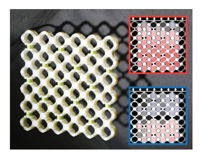
The metamaterial on the left offers multiple functionalities by changing its deformation. By compressing it slowly (bottom right) or fast (top right), we can change whether the metamaterial shrinks or expands when compressed. Credit: University of Amsterdam
