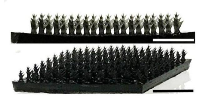
Images of representative fabricated PVA/PPy gel micro-tree array. Scale bar: 1 cm. Credit: California Institute of Technology
