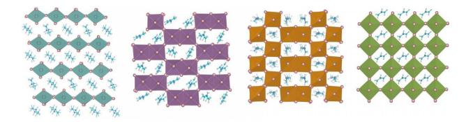
Researchers found that transformation from the intercalated initial structure to the final perovskite arrangement takes place via a sequence of intermediates. Credit: Ahlawat Paramvir, EPFL
