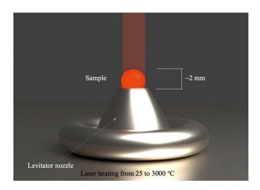
Illustration of the aerodynamic levitation process for studying refractory oxides at their melting points at the APS. A small bead of material is buoyed by gas and heated up by an overhead laser before X-rays examine its structure. Credit: Ganesh Sivaraman/Argonne National Laboratory.
