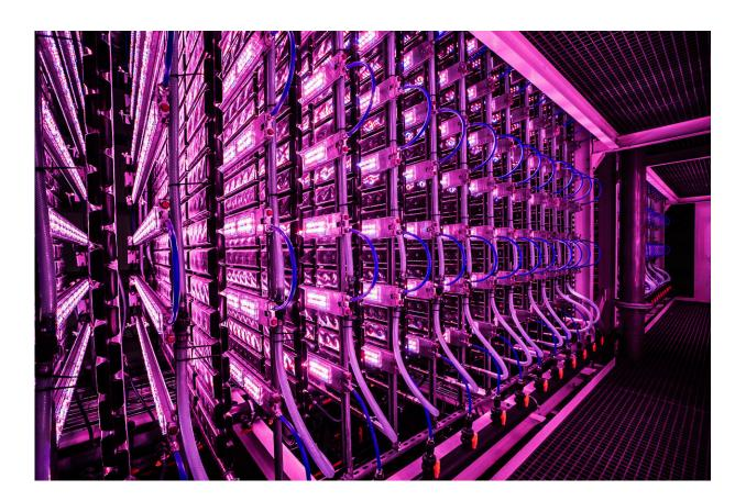
State-of-the-art, enclosed and modular photo-bioreactors (PBR) to produce chlorella and spirulina algae. Credit: Vaxa, Iceland.
