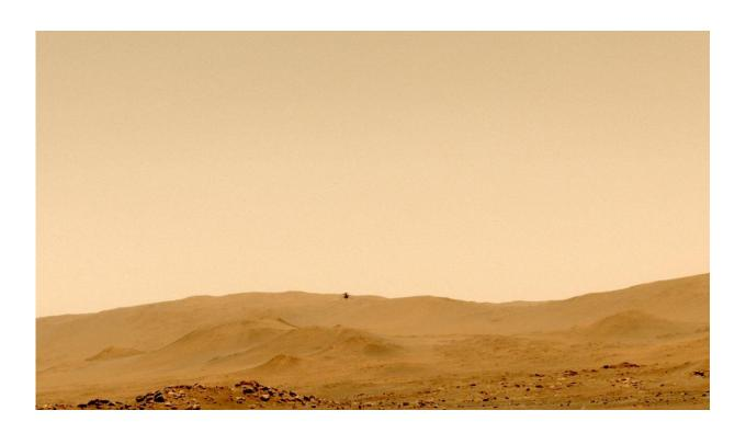
NASA's Ingenuity Mars Helicopter's fifth flight was captured on May 7, 2021, by one of the navigation cameras aboard the agency's Perseverance rover. The helicopter ascended to a new height record of 33 feet (10 meters) flew 424 feet (129 meters) to a new landing site. This was the first time the helicopter made a one-way flight. It was airborne a total of 108 seconds. Credit: NASA/JPL-Caltech
