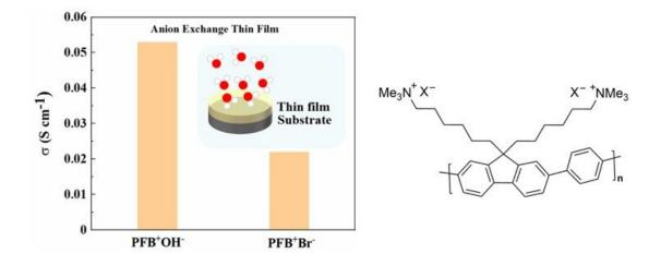
Figure 1: The first measurement of hydroxide conductivity and comparison in anion conducting polymer thin films. (X = OH and Br). Credit: Japan Advanced Institute of Science and Technology
