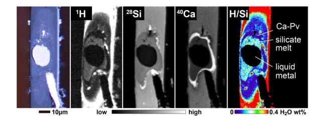
Sample from high-pressure experiment. High-resolution chemical analyses with secondary ion mass spectroscopy showed the abundance of water left in silicate melt after compressing with liquid iron metal. Credit: Tagawa et al.
