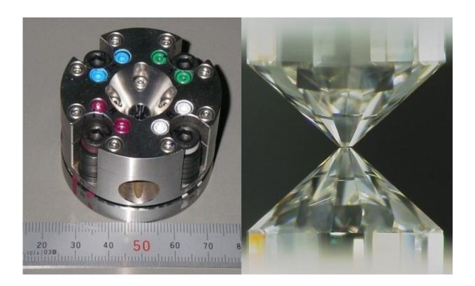
Diamond anvil. The outer metal casing and inner diamond teeth of the highpressure anvil. Credit: Hirose et al.
