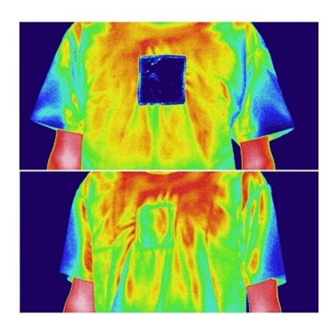
Thermal imaging shows how a square of the new textile (dashed lines) traps heat in heating mode (top), while reflecting it in cooling mode (bottom). Credit: Adapted from *Nano Letters*
