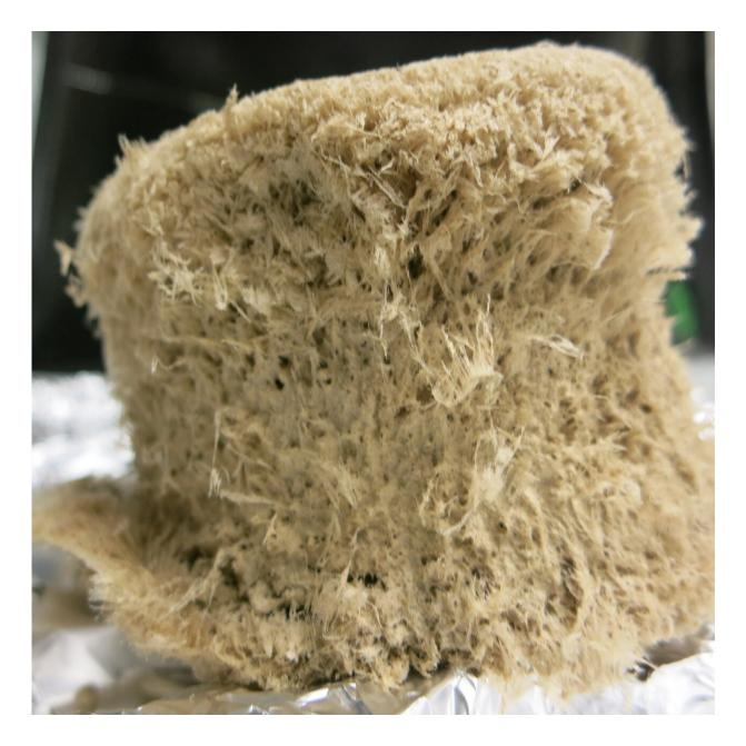
The production of bio-based materials (pictured here: foam made from microfibrillar cellulose) is the focus of research interest at the Institute of Bioproducts and Paper Technology. Credit: © TU Graz / BPTI
