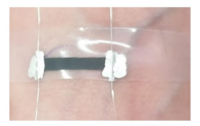
The team developed a method to formulate G-putty-based inks that can be printed as a thin-film onto elastic substrates, including band-aids, and attached easily to the skin. Credit: Trinity College Dublin
