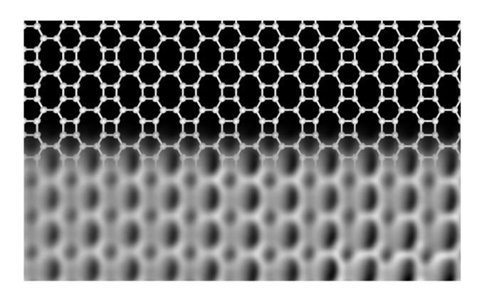
Structure of the new carbon network. The upper part shows schematically the linking of the carbon atoms, forming squares, hexagons, and octagons. The lower part is an image of the network, obtained with high-resolution microscopy. Credit: University of Marburg, Aalto University
