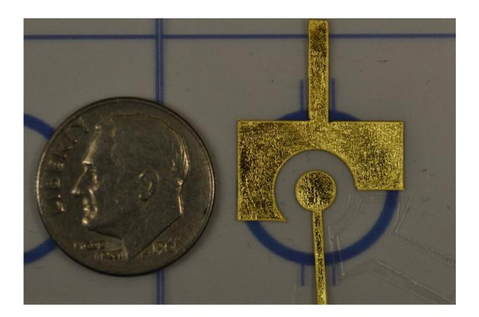
An inexpensive electrode made from gold leaf could be used to help detect viral infections in low-resource settings; a dime (left) is shown for size comparison. Credit: Adapted from *ACS Central Science* 2021, DOI: 10.1021/acscentsci.1c00186
