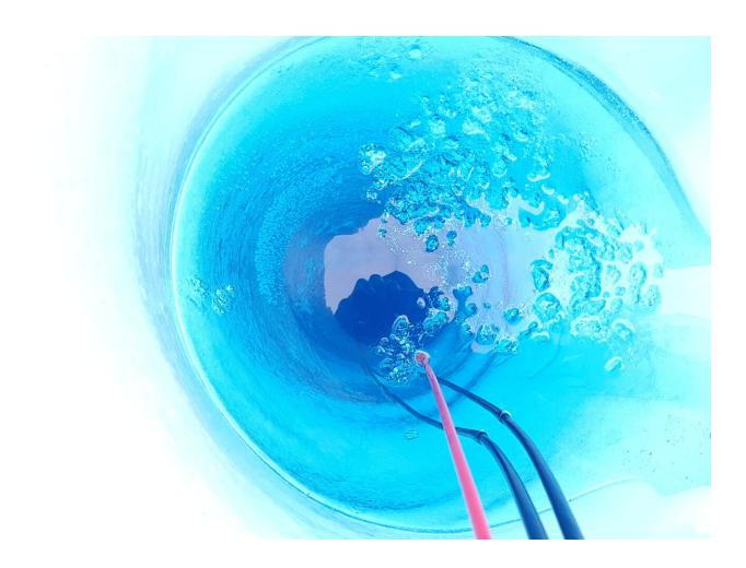
Fibre-optic cable (red) installed in 1 km deep borehole drilled on Store Glacier in Greenland. Credit: Poul Christoffersen and RESPONDER team
