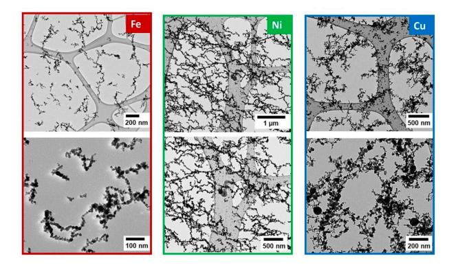
Image showing the stringlike particles formed by iron and nickel and the more globular clusters formed by copper. Credit: Abbaschian, Zachariah, et. al. 2021
