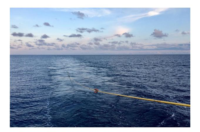
A special kind of antenna used to image the Earth like an ultrasound scanner trails behind the research vessel Marcus Langseth. Seismic investigators at University of Texas Institute for Geophysics used supercomputers at the Texas Advanced Computing Center Seismic to analyze a seismic image of a subduction zone in precedented detail. Credit: UT Jackson School of Geosciences/UTIG
