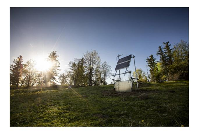
An upgraded Pacific Northwest Seismic Network monitoring station in Enumclaw, Washington, on April 20, 2021. The newly installed solar panels provide power for the system that detects the first signs of an earthquake. Credit: Mark Stone/University of Washington
