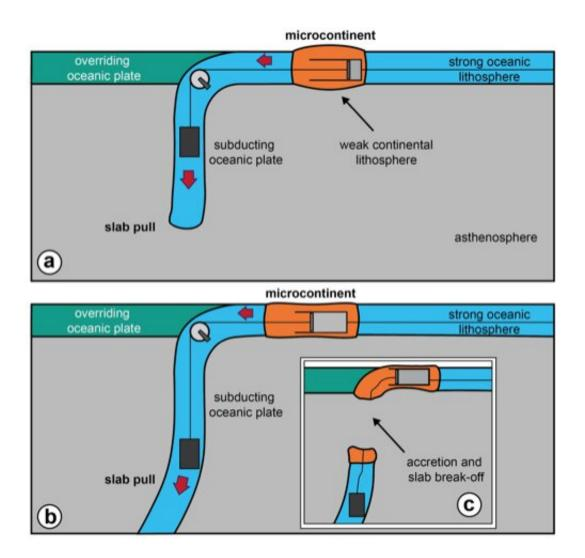
Elements of a newly discovered process in plate tectonics include a mass (rock slab weight), a pulley (trench), a dashpot (microcontinent), and a string (oceanic plate) that connects these elements to each other. In the initial state, the microcontinent drifts towards the subduction zone (Figure a). The microcontinent then extends during its journey to the subduction trench owing to
