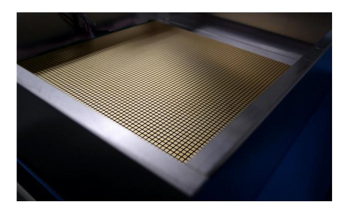
A LArPix sensor with 4900 pixels under testing at Berkeley Lab before shipment to the University of Bern for installation. Credit: Thor Swift, Berkeley Lab
