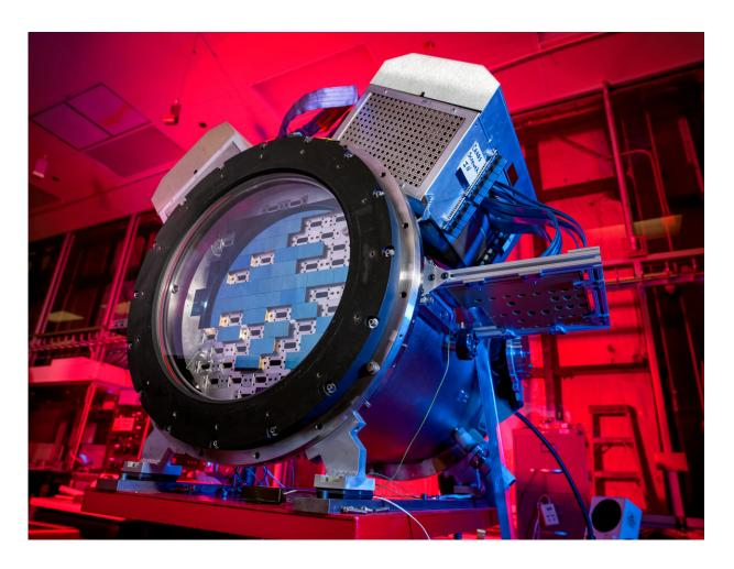
The Dark Energy Survey camera (DECam) at the SiDet clean room. The Dark Energy Camera was designed specifically for the Dark Energy Survey. It was funded by the Department of Energy (DOE) and was built and tested at DOE's Fermilab, Credit: DOE/FNAL/DECam/R, Hahn/CTIO/NOIRLab/NSF/AURA
