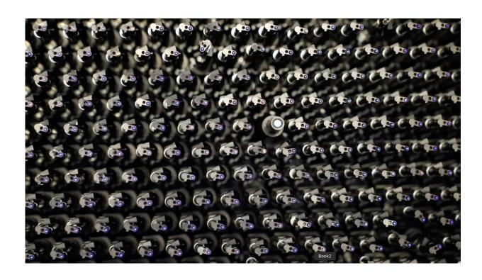
A small section of the DESI focal plane, showing the one-of-a-kind robotic positioners. The optical fibers, which are installed in the robotic positioners, are backlit with blue light in this image. Credit: DESI collaboration
