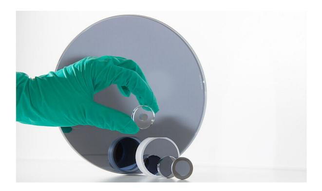
Crystalline interference coatings bonded on different optical substrates. Credit: Georg Winkler, Universität Wien
