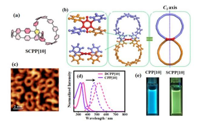
Structure (a) and theoretical calculating models (b) of SCPP[10]. STM image (c) shows Siamese-twin shaped structure of SCPP[10]. UV-vis absorption and fluorescence spectra of [10]CPP (the nanoring component of SCPP[10]) and SCPP[10] is shown in (d) and two molecules under UV irradiation at 365 nm. Is shown in (e). Credit: ZHANG Xinyu et al.
