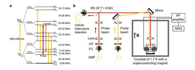
Energy level diagram and experimental setup. Credit: MA Yu et al.
