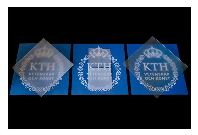
Previous versions of the see-through wood developed at KTH, left, are seen together with the latest, more translucent type developed with citrus derivatives. Credit: Céline Montanari
