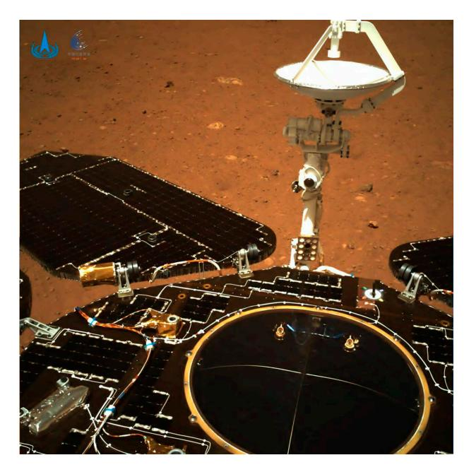
In this photo taken by China's Zhurong Mars rover and made available by the China National Space Administration (CNSA) on Wednesday, May 19, 2021, the rover's solar panels and antenna are deployed as the rover sits on its lander on the surface of Mars. China landed a spacecraft on Mars for the first time on Saturday, a technically challenging feat more difficult than a moon landing, in the latest step forward for its ambitious goals in space. Credit: CNSA via AP
