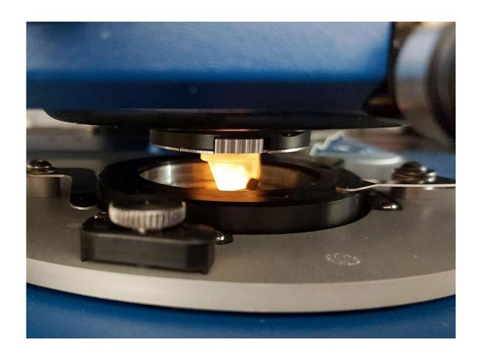
Element with a sampling probe (highlighted) in the atomic force microscope (AFM) at the Spectroscopic Imaging Laboratory of the Institute of Nuclear Physics, Polish Academy of Sciences. Credit: IFJ PAN
