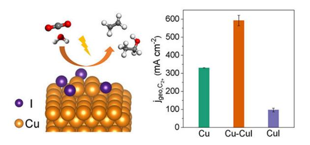
A Cu-CuI composite catalyst achieves highly efficient production of  $C_2^+$  chemicals from electrocatalytic  $CO_2$  reduction. Credit: LI Hefei and LIU Tianfu
