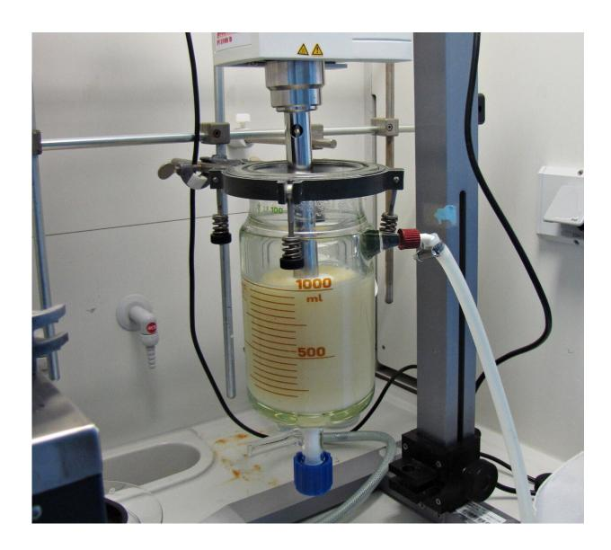
Fig. 3 The skill is in producing the aqueous coating dispersion in the correct mixing ratio of waxes, proteins and additives, as well as the sequence in which they are added. Credit: Fraunhofer
