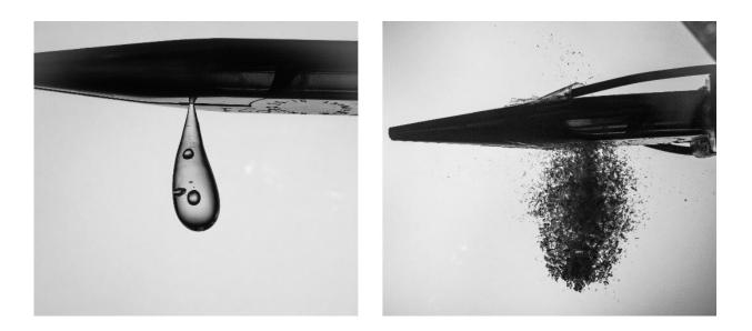
Left: a Prince Rupert's drop. Right: when the tail of the drop is squeezed, it breaks into countless tiny fragments – all roughly the same size. Credit: S. Kooij et al., Nature Communications
