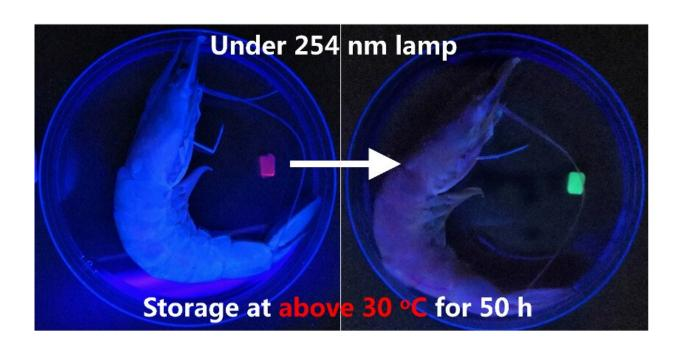
The color change of the "chameleon skin" hydrogel-based chemosensor in response to biogenic volatile amine vapors, which are a well known indicator of fish and shrimp spoilage. Credit: Lu et al./Cell Reports Physical Science
