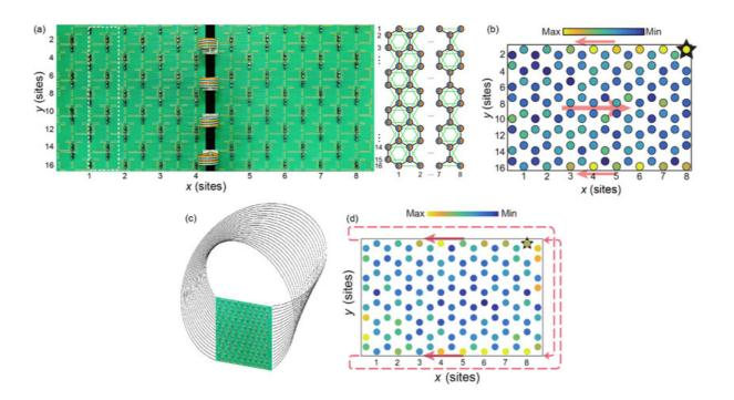
(a) Photo of electric circuit in experiments. (b) The measured antichiral edge states. (c), (d) A Möbius strip configuration consisting of electric circuit and the propagation of antichiral edge states in experiments, respectively. Credit:@Science China Press
