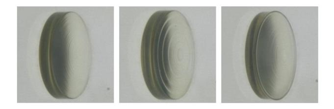
Researchers used 3D printing to make highly precise and complex apochromatic miniature lenses that can be used to correct color distortion during imaging. Credit: Michael Schmid, University of Stuttgart
