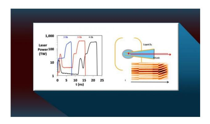
hese images depict various laser profiles used in the inertial confinement fusion research and provides the experimental set-up for the VISAR-based shock velocity measurement and representative streaked data. Credit: Lawrence Livermore National Laboratory
