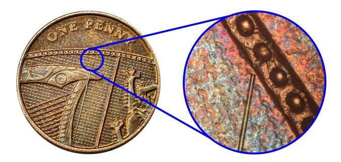
The optical fibre imaging sensor has a diameter of 125 micrometres, approximately the size a human hair, shown for perspective against a penny. A microscope image shows the true scale of the device, and its ability to conduct light. Credit: University of Nottingham
