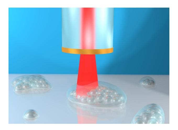
Concept art showing the 3D mapping of microscopic objects by the phonon probe system. The optical fibre contains a metal layer on its tip and projects red laser light into the specimen. Credit: University of Nottingham
