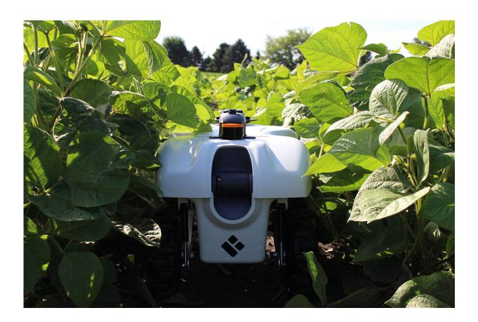
Researchers at the University of Illinois Urbana-Champaign have developed small-scale robots that can fertilize, weed and cull single plants in a field. This photo shows testing in an Iowa State University soybean plot. Credit: Photo by Ashlyn Rairdin and courtesy of Soumik Sarkar/Iowa State University
