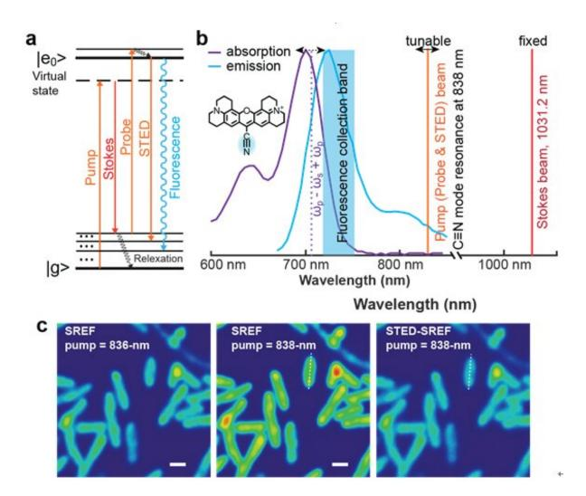
a, Energy diagram of STED-SREF. b, Spectroscopy configuration of STED-SREF. The nitrile mode of Rhodamine 800 (Rh800) is used here. c, SREF/STED-SREF imaging of Rh800 stained E. coli cells with pump wavelengths set at 836 nm (off resonance of the nitrile mode) and 838 nm (vibrational resonance of the nitrile mode). Direct coupling of stimulated emission depletion (STED) with SREF imaging fails to achieve desired
