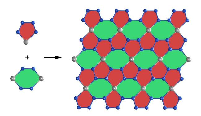
A single beryllonitrene layer consists of  $BeN_4$  pentagons and  $Be_2N_4$  hexagons. The beryllium atoms are shown as grey balls, nitrogen atoms as blue balls. Credit: M. Bykov
