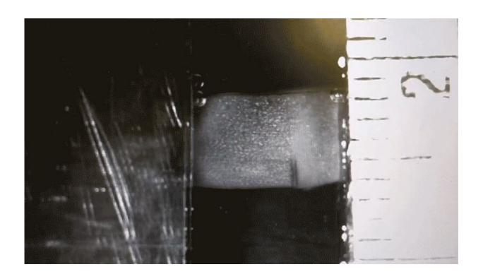
A steel particle is shown piercing through the nanofibrous hydrogel and exiting at a reduced velocity. The difference in velocity before and after gave the researchers a direct measurement of the material's impact resistance, or the amount of energy it can absorb. Credit: Jiahua Ni, Shaoting Lin, Xuanhe Zhao, et al
