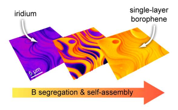
Studying the kinetics of borophene formation in low energy electron microscopy shows that surface steps are bunched during the borophene formation, resulting in elongated and extended borophene domains with exceptional structural order. Credit: *ACS Nano* (2021). DOI: 10.1021/acsnano.1c00819
