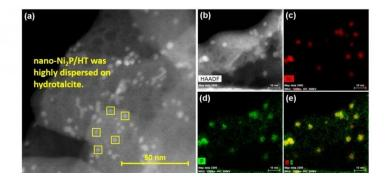
(a,b) High-angle annular dark field scanning transmission electron microscope image of nano- $N_2P/HT$ ; elemental mapping of (c) Ni and (d) P, and (e) composite overlay of Ni and P. Credit: Osaka University
