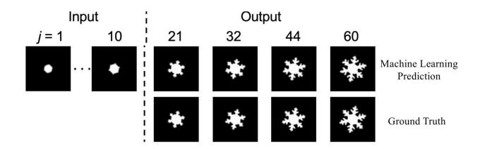
Engineers at Rice University and Lawrence Livermore National Laboratory are using neural networks to accelerate the prediction of how microstructures of materials evolve. This example predicts snowflake-like dendritic crystal growth. Credit: Mesoscale Materials Science Group/Rice University
